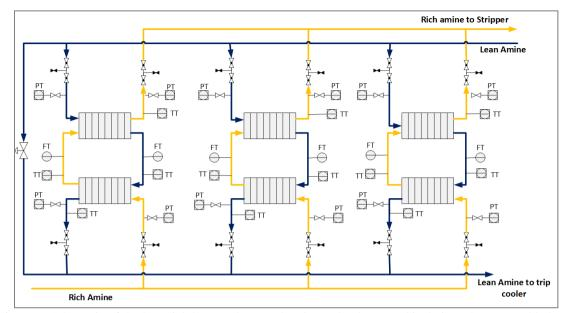
Figure 1. Schematic of the lean rich heat exchanger showing redundancy and isolations that were added
